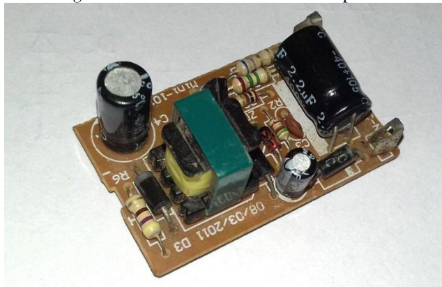
Fig 8. Power Supply Module
