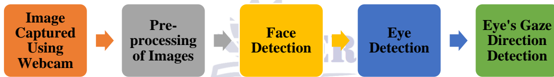
Figure 9: Proposed System Algorithm
