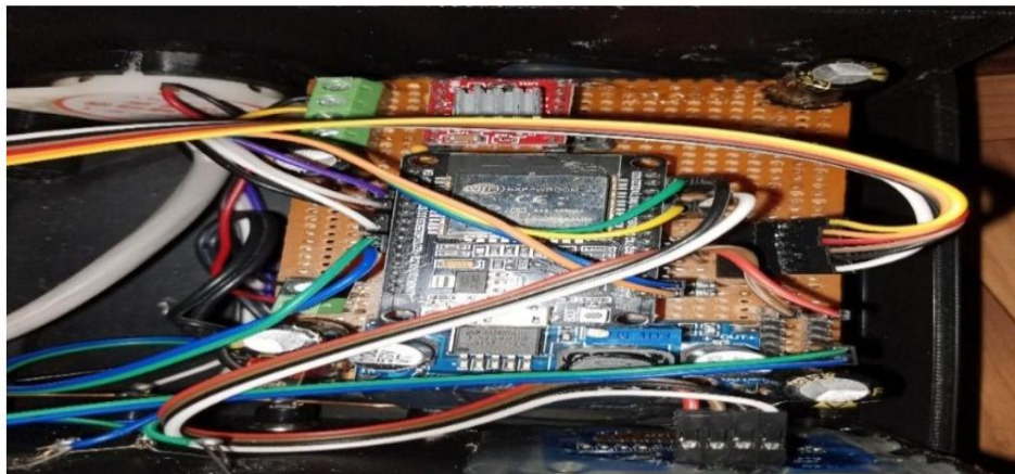
Fig 4-3: Solder components on vero board
