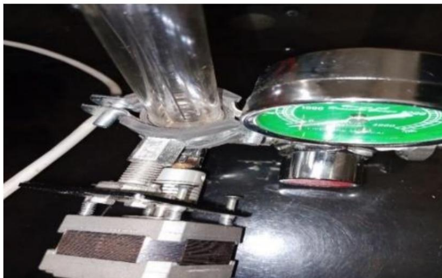
Fig 4-5: NEMA 17 motor attached with flowmeter valve using coupler
