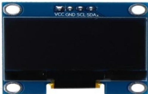
Fig 3-4: SH1106 1.3-inch OLED display
