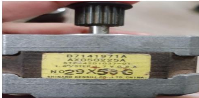
Fig 3-3: NEMA 17 stepper motor
